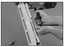
Figure 4. Loading nails into magazine.
